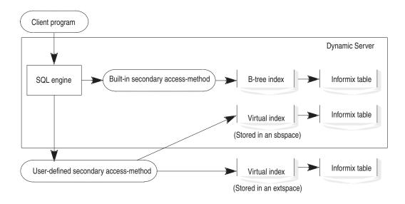
Figure 1-1. An Application Using a Secondary Access Method
