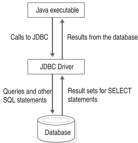
Figure 1-2. Runtime Architecture for Embedded SQLJ Programs
