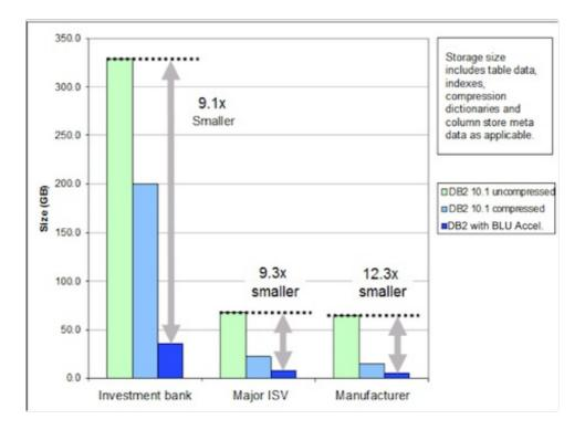
*Figure 2.* BLU Acceleration dramatically reduces storage requirements for analytics databases, typically by 10 times compared to uncompressed data in traditional databases.
